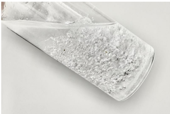
Fig 6 Phosphorus trioxide structure. The compound P 2 O 5 (more precisely P 4 O 10 ) has the same structure, but with four extra oxygen atoms at the phosphorus corners sticking out. Right: phosphorus trioxide solid and liquid at 23 °C.
